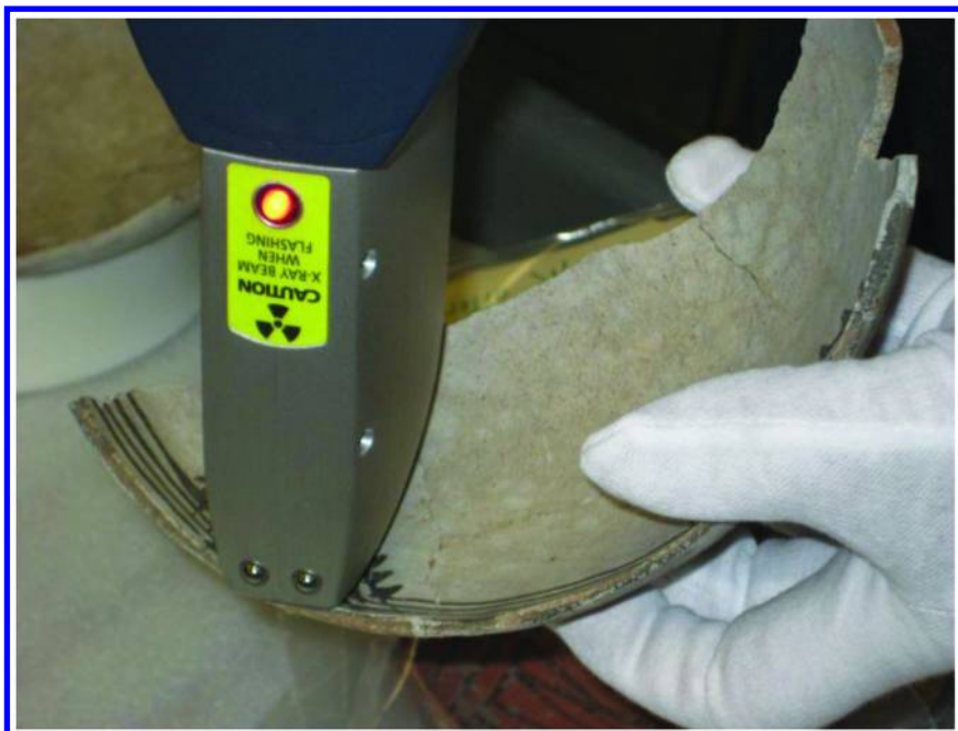
Figure 1. A photograph showing analysis of black pigment painted on a white ceramic from the Colorado Plateau. Readout indicated the presence of Pb and As in the pigment. That As was typical of all ceramics where Pb was indicated as a major component of the pigment. That is, in every case when high levels of Pb were recorded, lesser amounts of As were also reported on by the pXRF.
