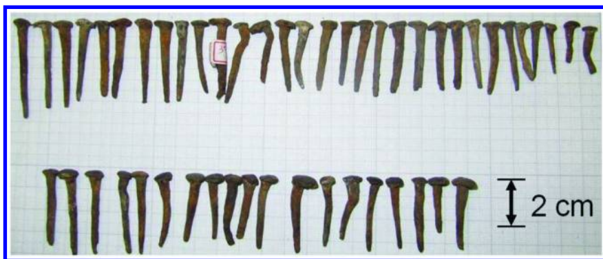
Figure 12. Iron nails used for the woodblocks.
