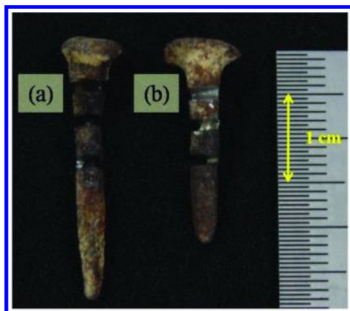
Figure 13. Nails were cut cross section and longitudinal direction.
