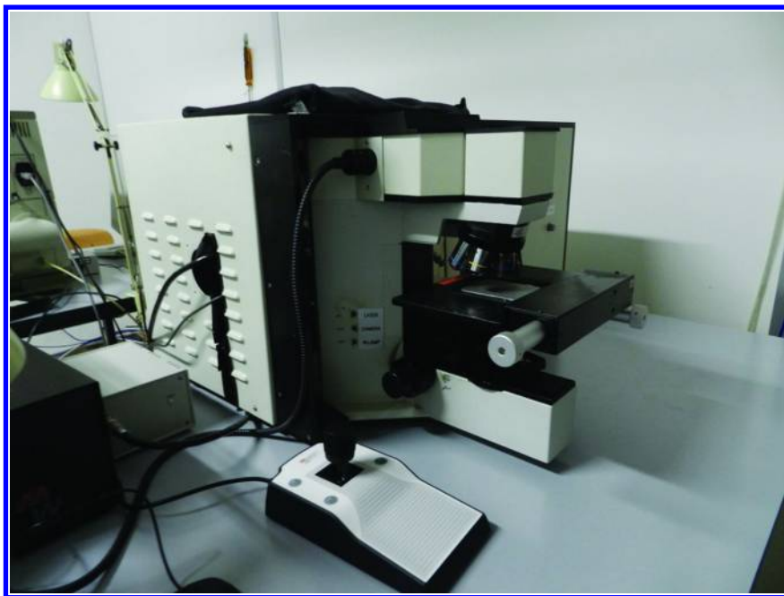
Figure 6. A typical RM Spectrometer (Horiba LabRAM) equipped with EDGE filters, 10, 50 and 100X objectives and telecamera. Courtesy of the University of Modena and Reggio Emilia, Italy. Photograph: M. V. Orna.
